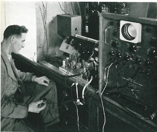
Above (left): Testing a lamp subsequently used for photographing the retina of the human eye. It is a low power lamp which can be focused on the retina and pulsed to a very short brilliant flash for the photograph. (right): Mazda electronic flash tubes. Background: Rare-gas flash tubes enable the photographer to capture movements which are invisible to the human eye.
