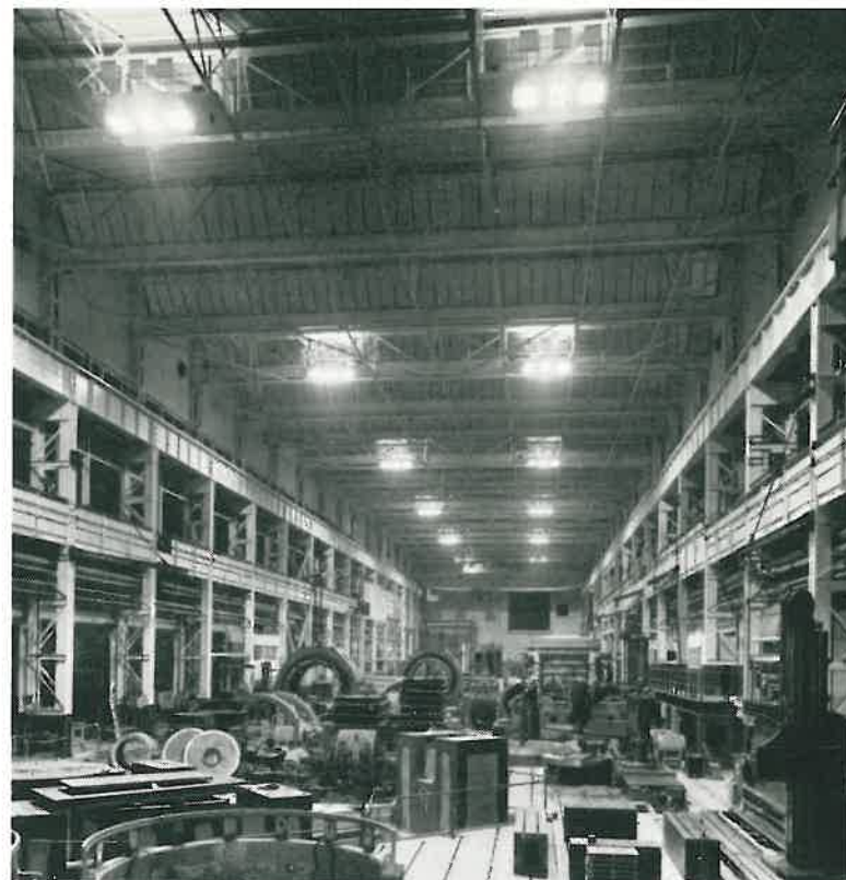
An experimental installation of Mazda 2½-kW mercury discharge lamps used in combination with tungsten lighting during 'field' trials in an engineering workshop. This research led to the development of the Mazda 1-kW MA|H lamp (see page 17).
